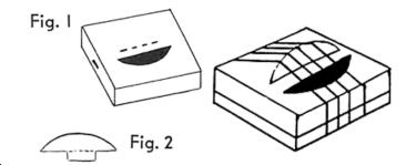
5cm in depth. Cut a hole and a slot in the cover, as pictured in figure 1. Cut out a bridge from cardboard, as in figure 2. Make certain that the tab at the bottom of the bridge fits securely into the narrow slot, and that the bridge stands upright. Return cover to box and secure with tape. Stretch rubber bands of various sizes over the entire box passing them over the bridge. The smaller bands which are stretched more tightly over the bridge will produce the highest tones.
